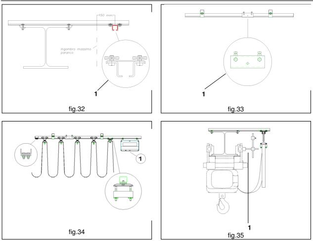
**§ Assembly of the rotating collector ring** (if installed):
