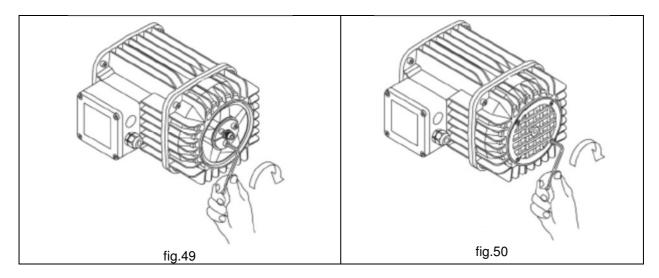
If the adjustment has been performed various times and it is not longer possible to obtained the desired braking, it is necessary to replace the motor cover ONLY order the original spare part.
